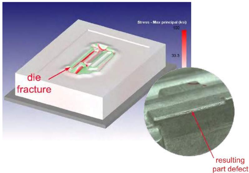
The crack resulted in a defect on the forging.
